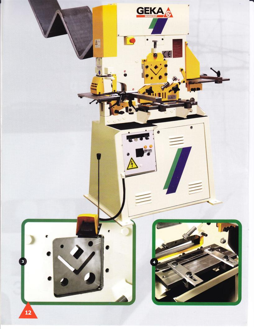
Metal fabricators and construction companies often have to perform simple bending operations. **GEKA** has developed the **BENDICROP** model which, apart from the cutting, punching and notching stations holds a permanently fitted bending station with a capacity of up to 4" x ³/8". Furthermore, it is fitted with a system to reduce deformation when shearing flatbar.
